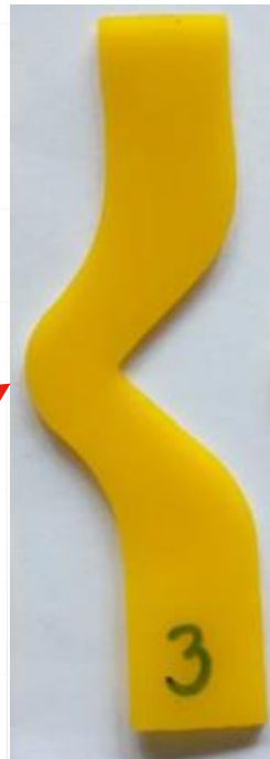
ASTM D412 – tensile test
