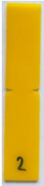
EWF-test (notch-razor sharpened crack like defect)
