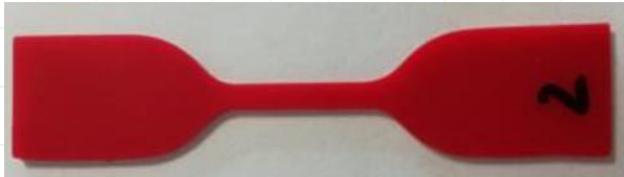
ASTM D412 – tensile test
